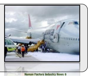
According to a probable cause report by the NTSB, the plane's flight crew failed to confirm there were five green landing gear indicator lights, as stated in the checklist. The crew instead made general comments about the lights, such as "got em all," the report states.
